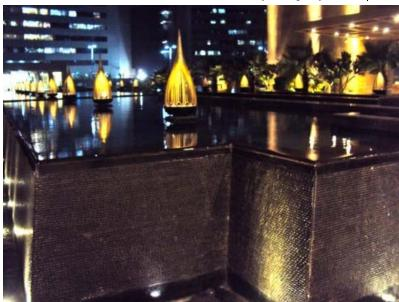
Hardscape and Water Features: The entrance driveway is cobbled in Black Granite & Yellow Jaisalmer hand-cut cobbles in  $200 \times 100 \times 100$  mm. A raised reflective water body is clad with Tropical Green Granite, which is grooved and chipped to provide a white water effect. Floating Lanterns on the reflective water body have a solid stone spherical base and brass tops. Tropical Green Granite sculptures of 1500 mm height and with a high gloss finish are placed in the alfresco dining area.
